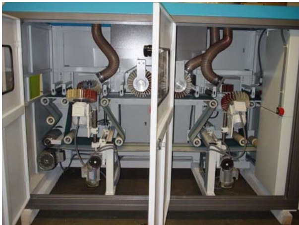
The inside of an LZ 3x2-300 with belt feed and hold down rollers shown left. Side heads shown right.
