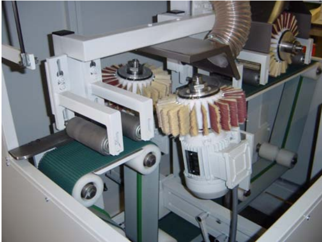
The inside of an LZ 3 with belt feed, hold down rollers and tilted heads shown left. Side heads shown right.
