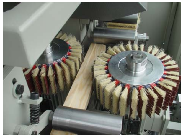
Upper and lower heads with belt feed and hold down rollers shown left. Side heads shown right.
